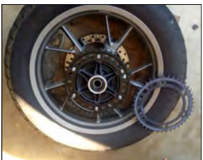
Rear wheel with old sprocket removed, new sprocket in place.
