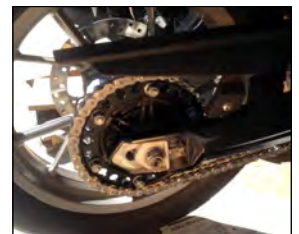
New chain and sprocket on and tension adjusted per the manual. Ready to ride.
