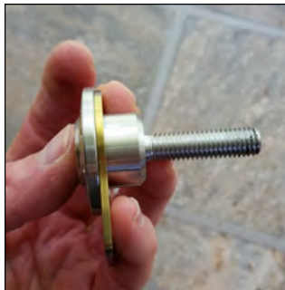
The bracket slid on the bolt that attaches it to the bike.
